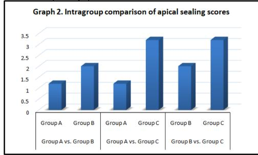
On comparing Group A (Endoseal MTA) and Group B (BioRoot RCS) the mean depth of dye penetration in Group A (Endoseal MTA) was 1.2mm and Group B (BioRoot RCS) was 2mm. The difference of which was statistically significant.
