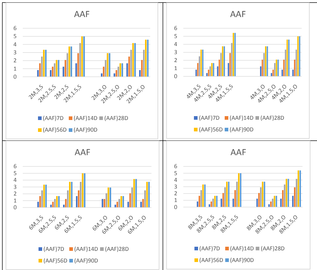
Fig: 2: AAF of Geopolymer Mortars 2,4,6,8M & NS/NH=1.5,2,2.5,3 for 7,14,28,56,90Days in Ambient(S) & Oven(O) in H_2SO_4
