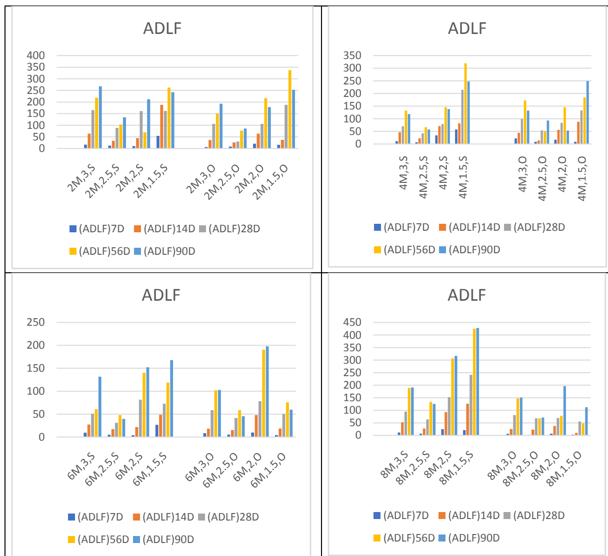
Fig: 4: ADLF of Geopolymer Mortars 2,4,6,8M & NS/NH=1.5,2,2.5,3 for 7,14,28,56,90Days in Ambient(S) & Oven(O) in H 2 SO 4
