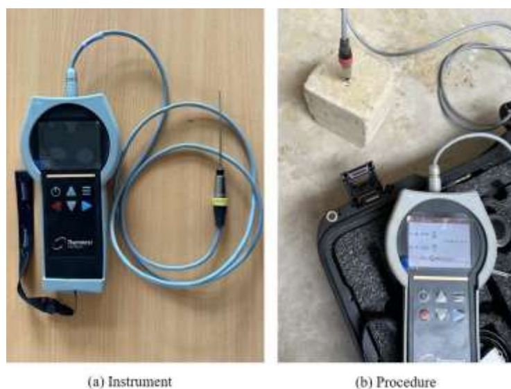
Fig. 4 Thermal Conductivity Coefficient Measurement Procedure
