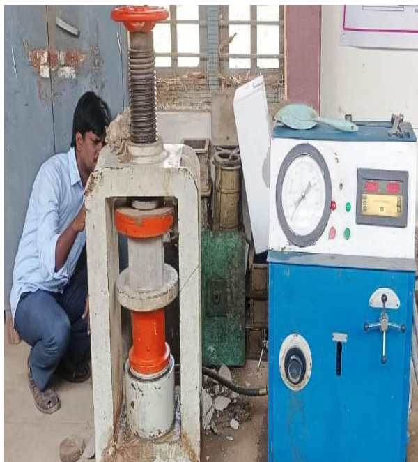
Figure 1. Testing the specimen for Compressive Strength.
