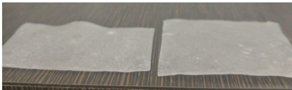
Fig. 1 2x2 cm 2 drug loaded transdermal patches
