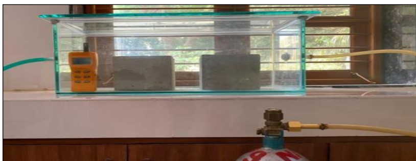
Fig 4. Experimental setup of CO 2 reduction test
