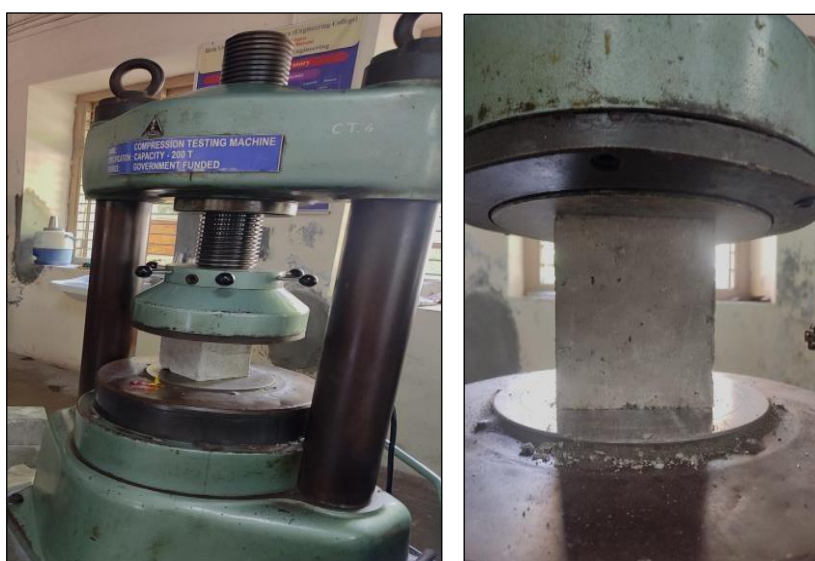
Fig 3. Compressive strength test
