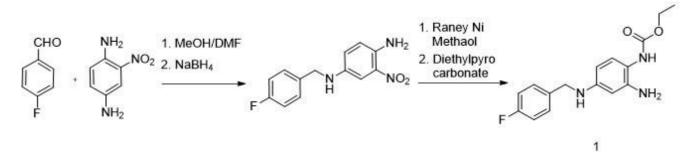
As mentioned in the scheme 1, synthetic process of Retigabine contains Methanol as a solvent. An inhouse HPLC method is developed to separate the related substances from Retigabine, and this method contains Acetonitrile solvent as Diluent and Mobile phase. In presence of Methanol and Acetonitrile solvents, these two impurities formation was observed.
