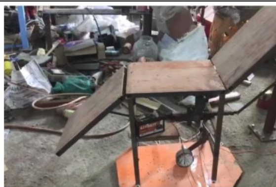
9.3.2 Wheel chair model with base, head rest and foot rest
