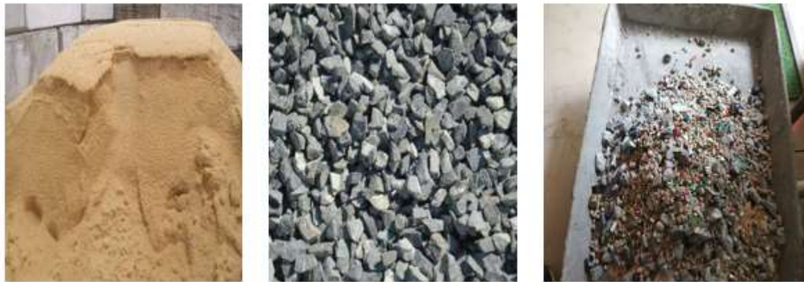
Figures 11, 12 & 13: Fine aggregates, Coarse aggregates, dry mix with E wastes
