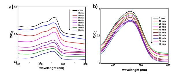
Fig. 7. Absorption spectrum of photodegradation of a) MB and b) MO dye under
