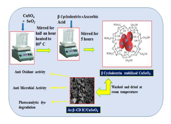
Fig 1: Schematic representation of biosynthesis of As: β–CDIC/CuSeO<sub>4</sub>
