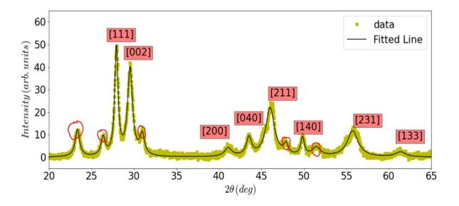
Fig.2.XRD patterns of as-synthesized As: β–CD IC/CuSeO<sub>4</sub>nanoparticles.
