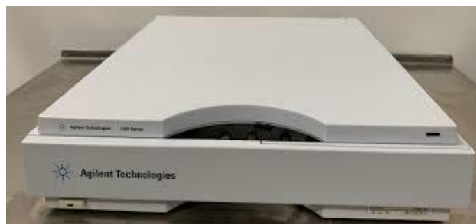
Figure 5. A micro-Degasser and its supplies which has a flow rate of up to 5ml/min and an internal volume of 1ml
