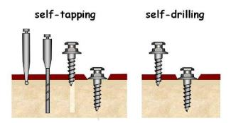
Figure 3: Self tapping and Self drilling screws
