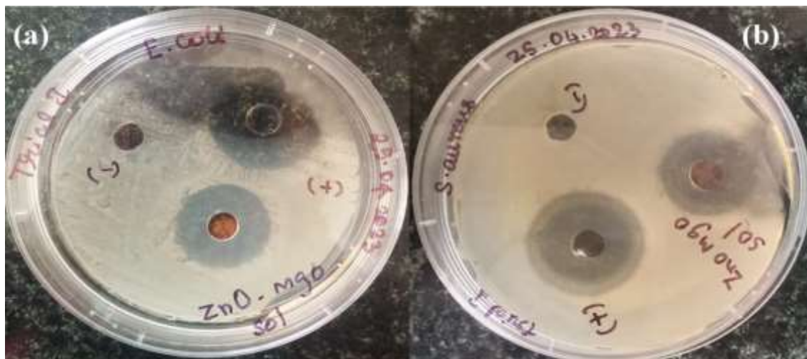
Fig.8: Antimicrobial activity of the mixture solvent mediated ZOMONC's sample versus (a) Escherichia coli and (b) Staphylococcus aureus
