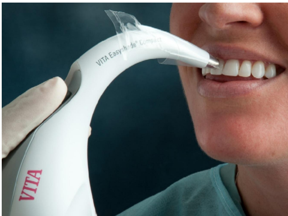
Figure 6: Colour measurement by spectrophotometer
