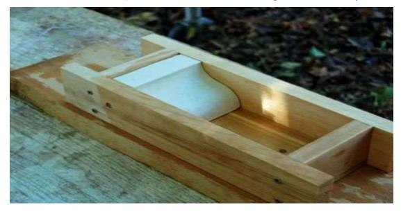
The plastic bricks were produced by mixing PET plastic waste with fine aggregate in various proportions. The mixtures were then moulded into brick shapes using a manual brick press. The bricks were then subjected to various tests, including compressive strength, water absorption, and weathering resistance tests. The results were recorded and analyzed.
