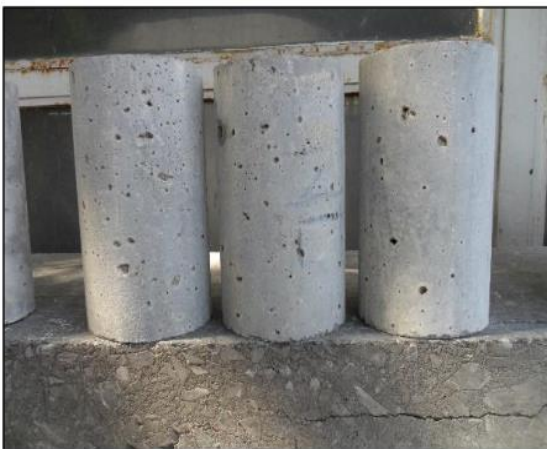
Figure 4. Surface Deterioration of HSNWC specimens stored in magnesium sulphate sol.
