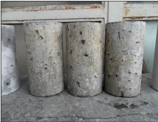
Figure 3. Surface Deterioration of HSLWC specimens stored in magnesium sulphate sol.
