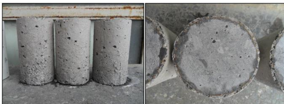
Figure 7. Surface Deterioration of HSLWC specimens stored in Sulphuric Acid sol.
