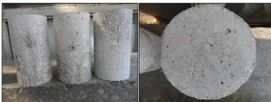
Figure 8. Surface Deterioration of HSNWC specimens stored in Sulphuric Acid sol.
