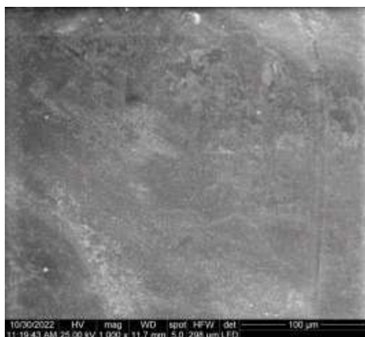
Figure (7): SEM photomicrograph (x1000) of nanofilled composite without any polishing protocol (control)
