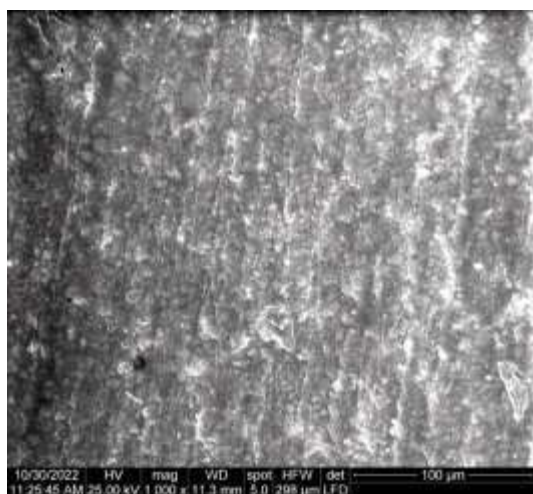
Figure (19): SEM photomicrograph (x1000) of nanofilled composite subjected to heavy then intermediate then light pressure in wet condition with coolant
