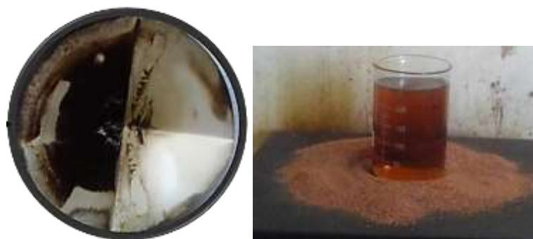
Figure 5: Separation of asphaltene and resins
