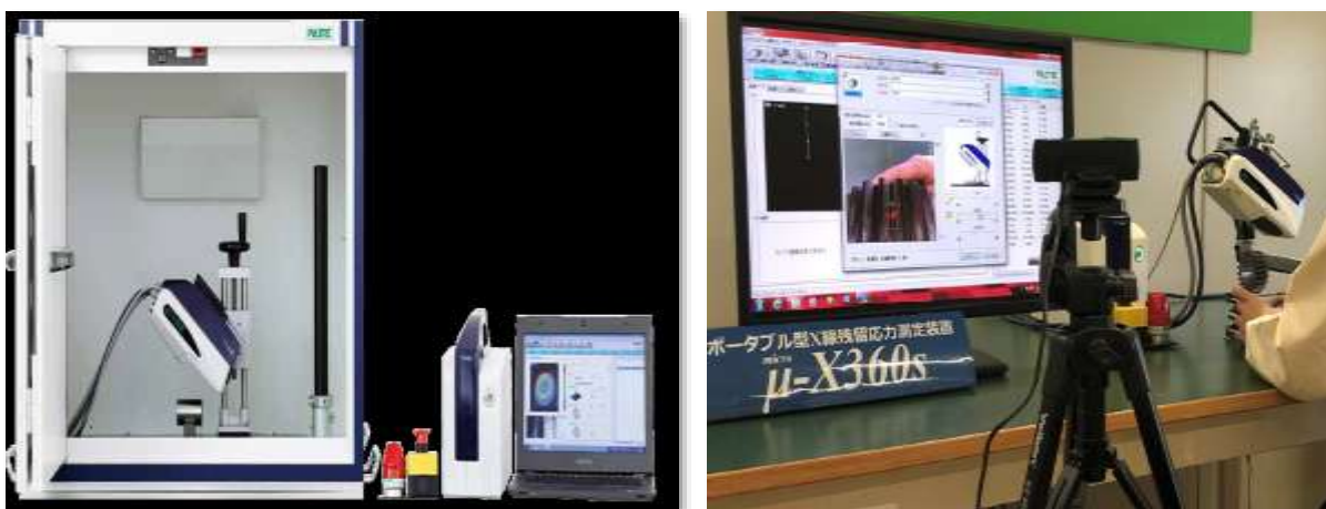
Fig.3 Components of Portable X-Ray Residual Stress Analyser Micro- \mu -360s
