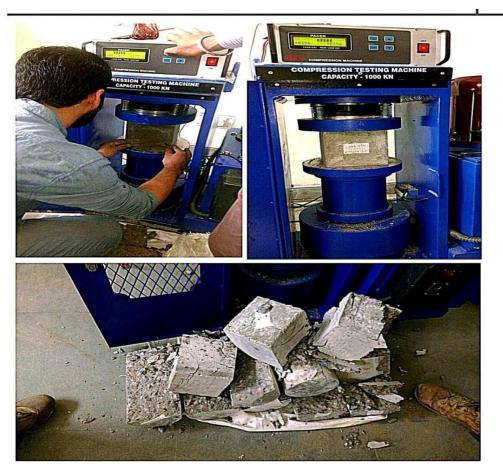
The results of compressive strength of cubes for (7, 28) days curing are shown in table. It should be noted that in mix M1, M2 and M3 compressive strength increases as the days of curing are increased from 7days to 28 days. But as the percentage replacement of quarry dust reaches the value 30%, compressive strength *1Eur. Chem. Bull.* **2023**, *12*(Special issue 4), *11048 – 11062*
