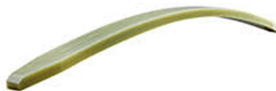
Fig (7.1): Prototype of composite leaf spring manufactured considering above obtained dimensions.
