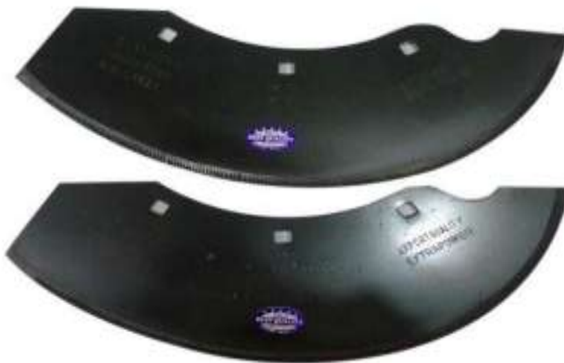
Fig No.2 Straight Rectangular Chaff Cutter Blade and Chaff Cutter Blades
