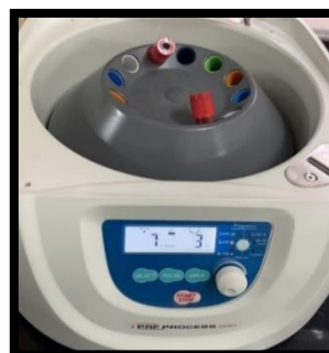
Fig 4: -I-PRF tubes placed in the Choukrons process for PRF centrifuge and centrifuged at 700 rpm for 3 mins
