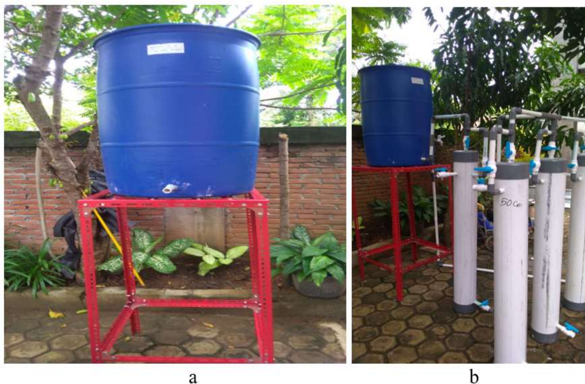
Figure 1: Water storage and coagulation (a. Water storage in tanks; b. Water filtration and coagulation construction)
