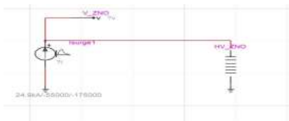
Fig 13. ZnO surge arrester energization.
