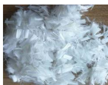
Figure 2: Novel Polypropylene Fiber
