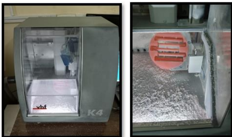
Fig. 4. Milling of CAD-CAM samples
