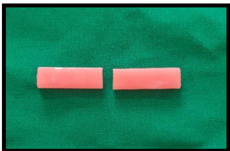
Fig. 9. Fractured PMMA sample
