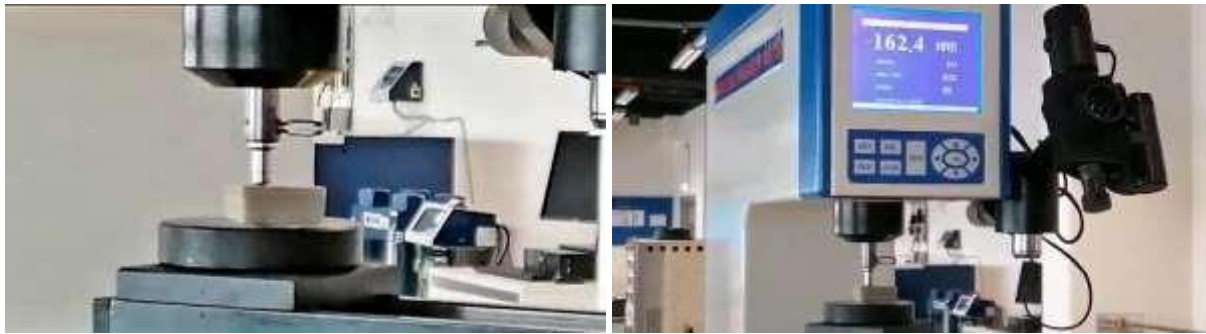
Fig 6: Brinell Hardness Test of Specimen I & Specimen II
