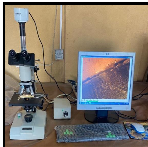
Figure (2) shows euromex microscope was used to measure the maximum border gap.
