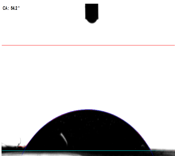
Fig 11c contact angle for 100 cycles of graphene-coated glass
