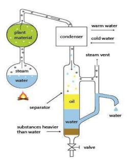
Figure-1. (a) Hydrodistillation-Clevenger method (b) Steam distillation method
