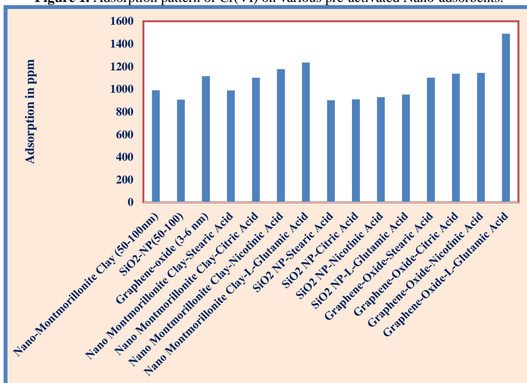
Figure 1. Adsorption pattern of Cr(VI) on various pre-activated Nano-adsorbents.
