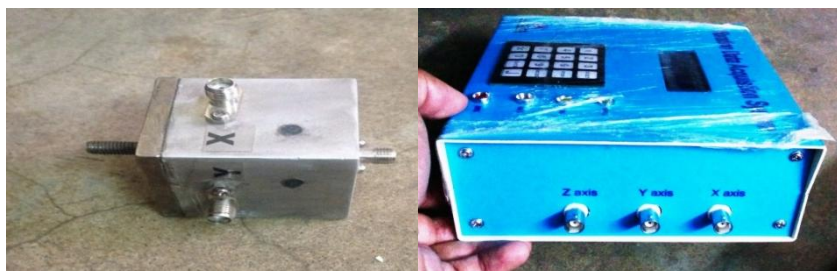
Figure2.3 Tri-axial Sensor and Data Acquisition unit setup used for the measurement of vibrations
