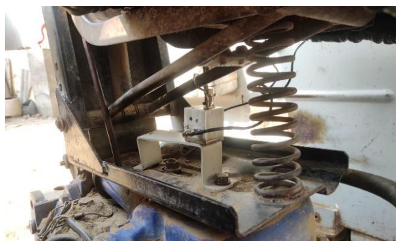
Figure 2.2 Location of tri-axial accelerometer on the base of tractor seat.
