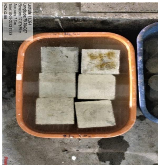
Fig. 14 Specimens immersed in solution ( H_2SO_4 )
