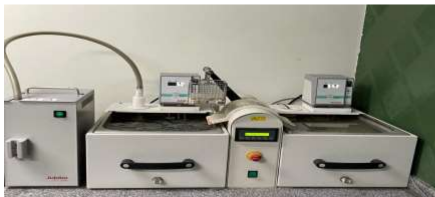
Figure 6: Thermocycling device (German-made 100 SD mechatronic thermocycler)
