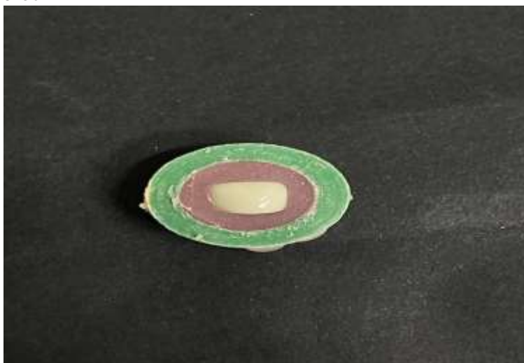
Figure 1: Embedding the crowns on an acrylic encircling a wax block
