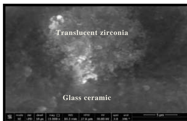
Figure (7): Representative SEM image x15000 magnification of de-bonded veneered translucent zirconia using Free-Hand Layering technique.
