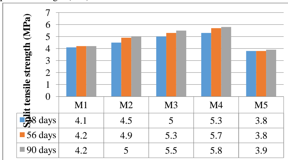
Figure 5 Split tensile strength of concrete at different curing days
