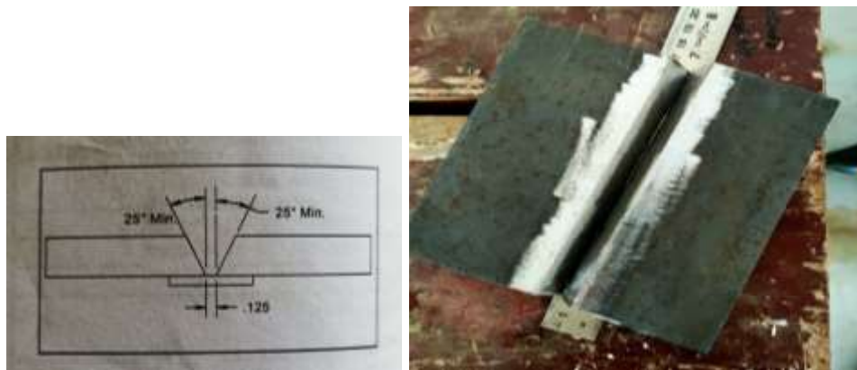
Figure 1: Experimental sample with V-type groove before welding.
