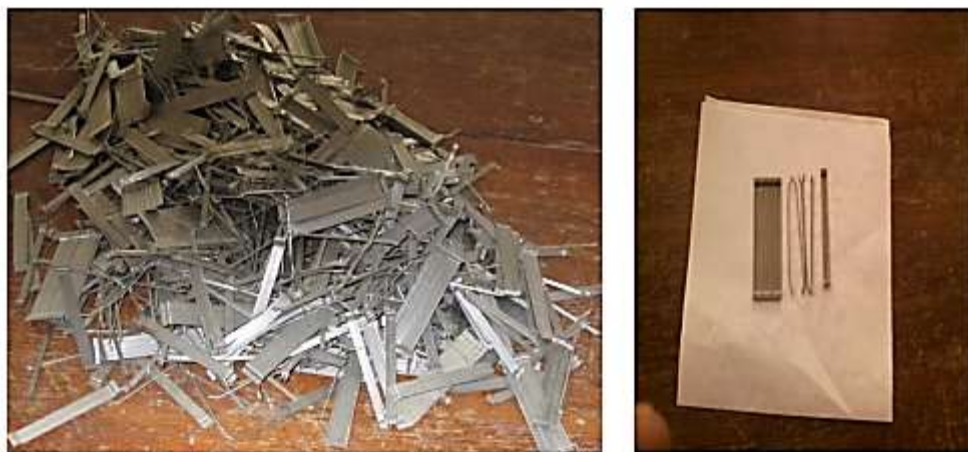
Figure 1(a) Steel fiber of aspect ratio 80
