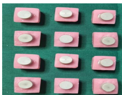
Fig.1 30% CARBON REINFORCED PEEK SPECIMENS
