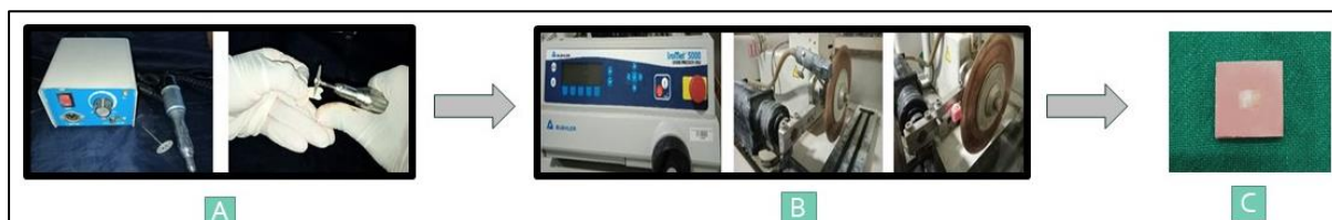
Figure 1: Sample preparation: A) Premolar tooth sectioned at the cemento-enamel junction. B) Proximal sections prepared with ISOMET 1000, USA. C) prepared section embedded in acrylic block
