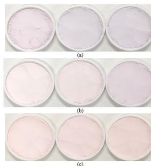
Figure 6. Photographs of precipitates II prepared under various conditions, from left, 1, 2, 3 times of acid quantity, (a) \text{HNO}_3 , (b) \text{HCl} , (c) \text{H}_2\text{SO}_4 .
