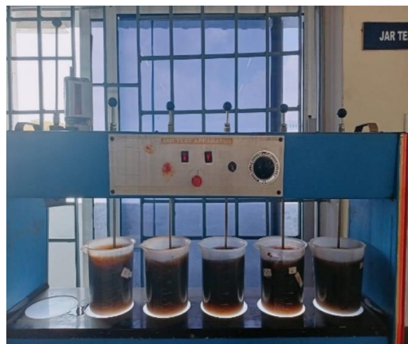
Fig 2. Coagulation flocculation of leachate
