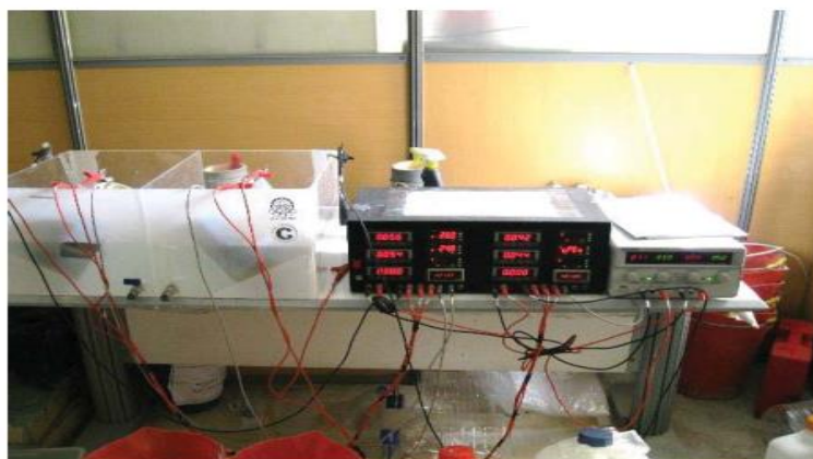
Figure 3.4. The equipment for measuring rapid chloride migration
