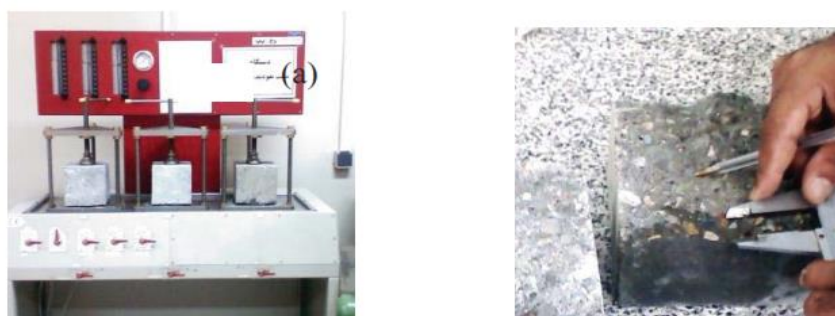
Figure 3.3. Measuring water penetration resistance: a) equipment b) test specimen
