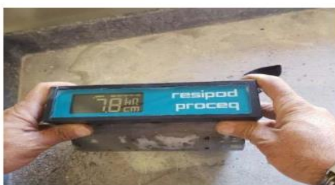
Figure 3.2. Measuring SER using 4-probe Wenner-array device
