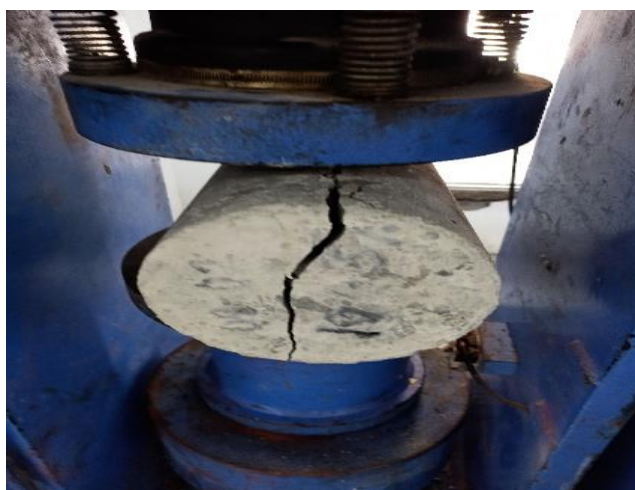
Figure 11: Testing of concrete cube specimen for tensile strength
