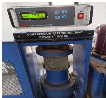
Figure 7: Testing of concrete cube specimen for compressive strength
