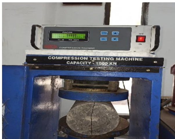
Figure 10: Testing of concrete cube specimen for tensile strength
