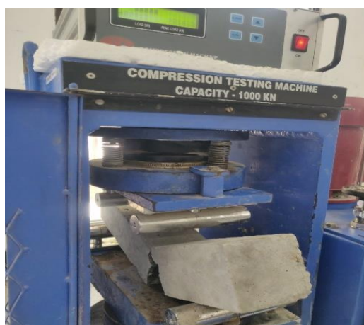
Figure 15: Testing of concrete beam for flexural strength
