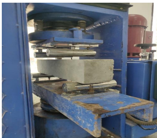
Figure 14: Testing of concrete beam specimen for flexural strength
