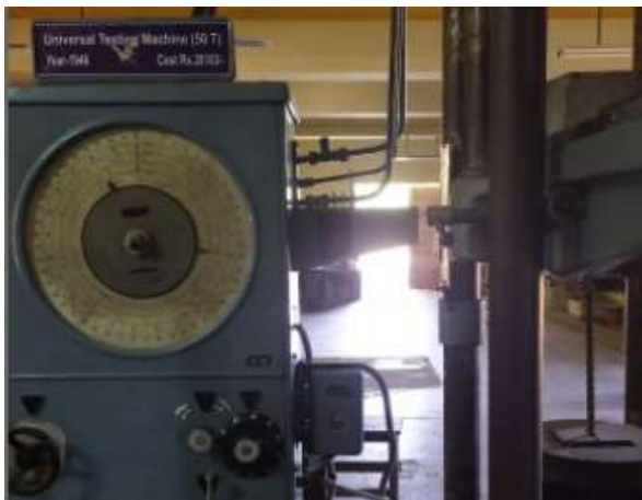
Figure 19. Pull out test setup
