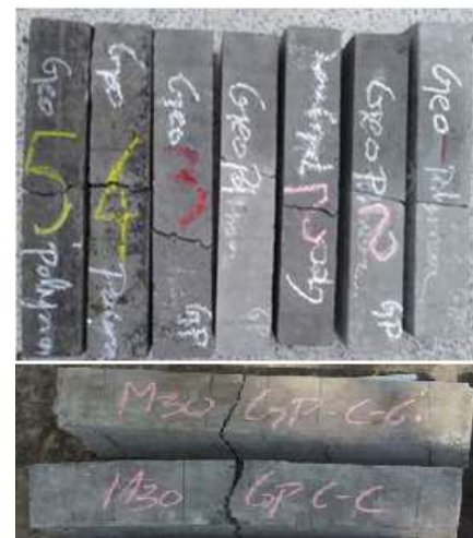
Figure 26. Failure of prism
