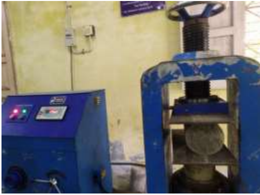
Figure 13. Testing of cylinder specimen
