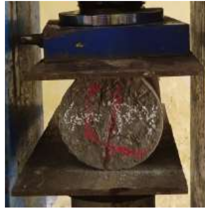
Figure 14. Failure of cylinder
