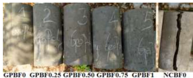
Figure 24. Failure of cylinder
