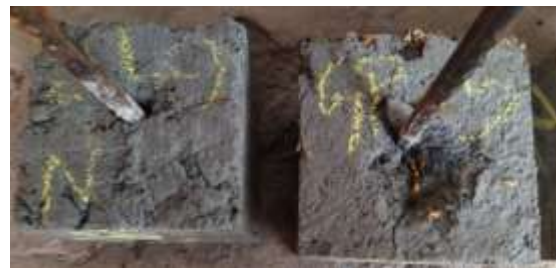
Figure 20. Failure of pull out specimen
