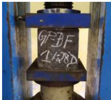
Figure 12. Failure of cube
