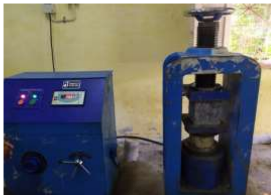
Figure 11. Testing of cube specimen
