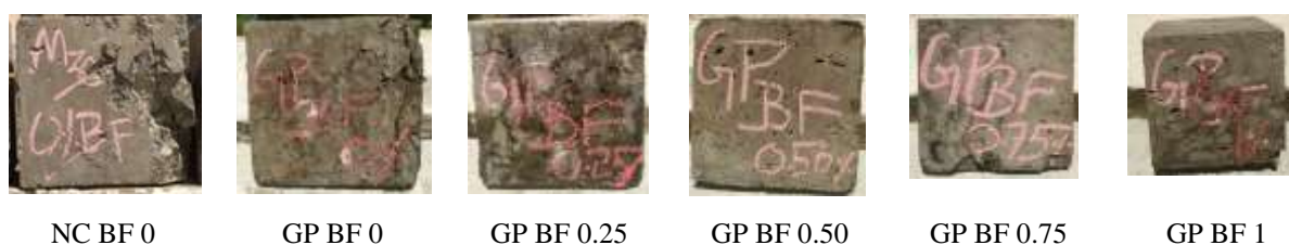
Figure 22. Failure of cube
