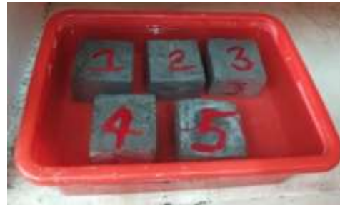
Figure 18. Water absorption test
