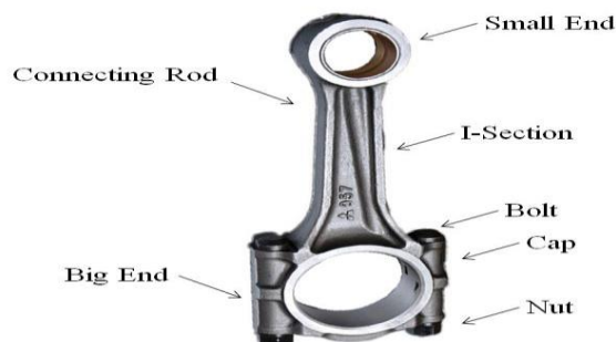
Figure 0.1: Schematic illustration of Connecting Rod
