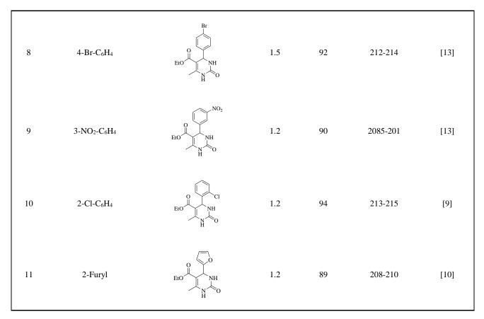
Yield of reactions using aldehyde (2 mmol), ethyacetoacetae (2mmol), urea or thiourea (3 mmol), nanocomposite ferrite (10 mol %) and 2 drops HCl in ethanol (5 mL) at 60 °C temperature.
