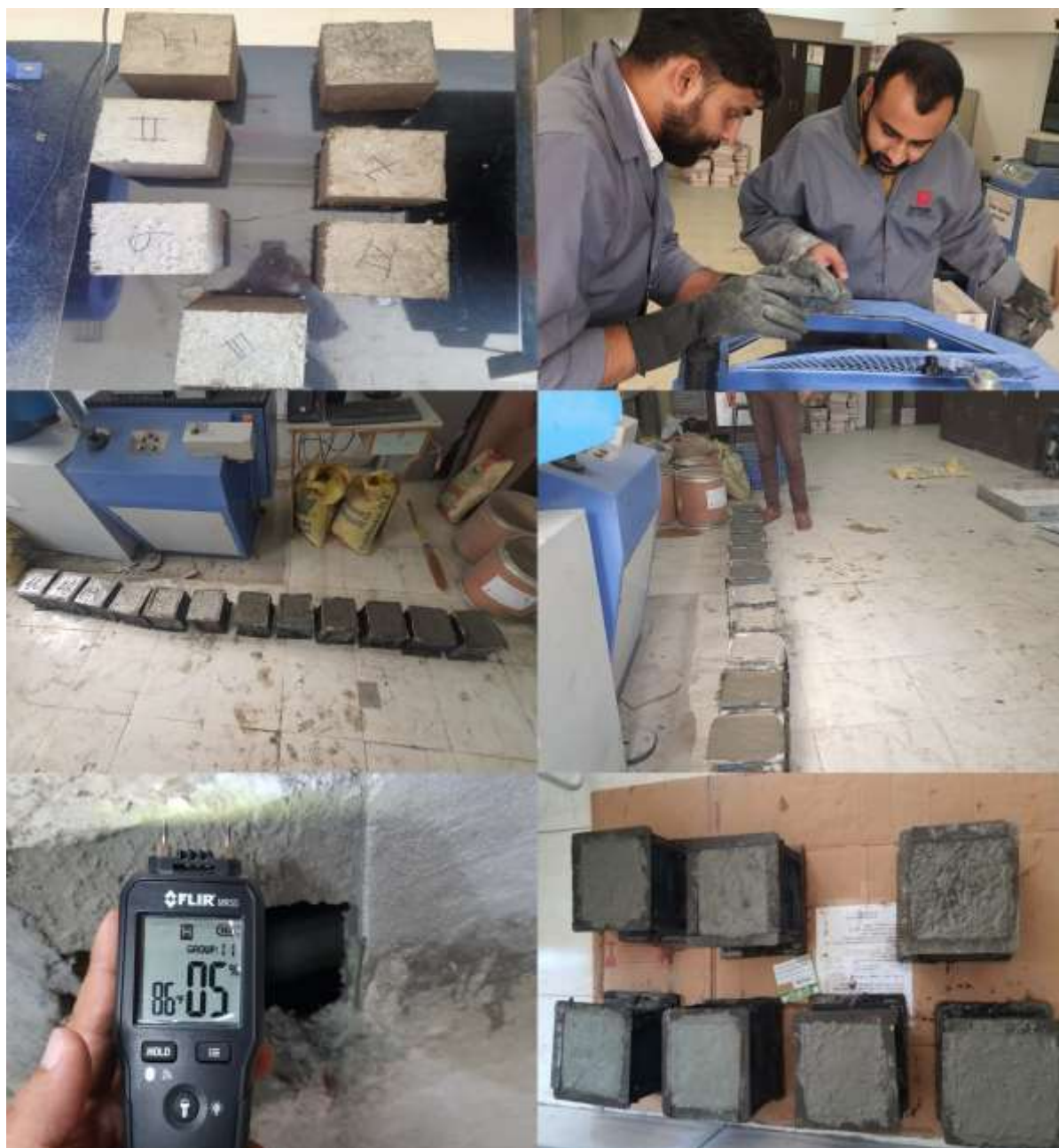
Fig. 9: Processing of Hemp Concrete Blocks and Moisture Content Measurement
