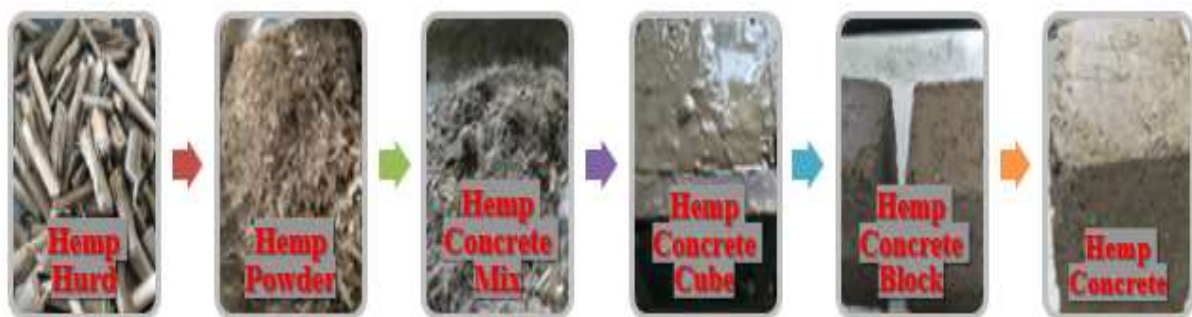
Fig. 8: Processing of Hemp Hurd and Concrete Blocks
