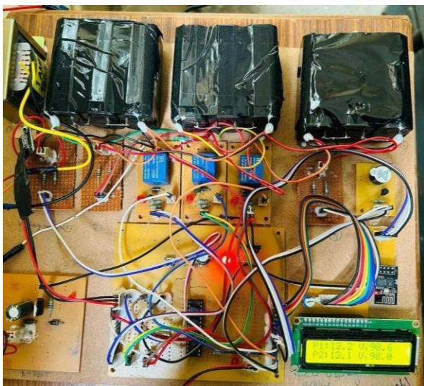
Fig.3. The Hardware kit of BMS and SOC development.
